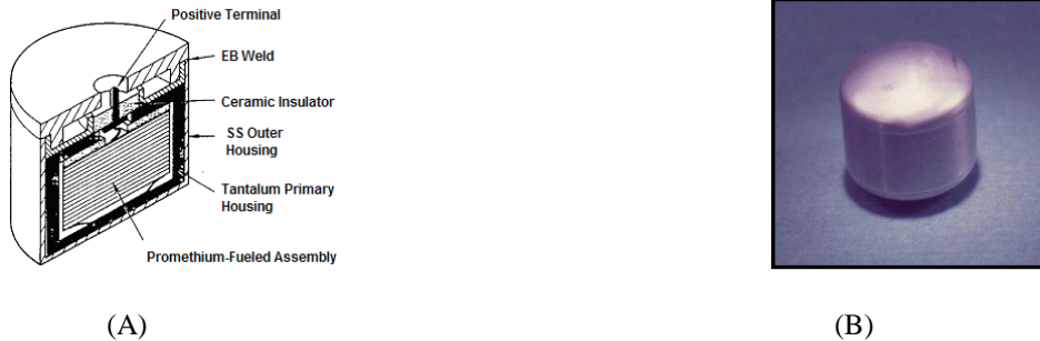
Figure 1. (A) Configuration used for Betacel batteries. (B) Picture of a Betacel battery that produced 400 \mu W. A large part of the total volume of approximately 1 in 3 was due to shielding.
